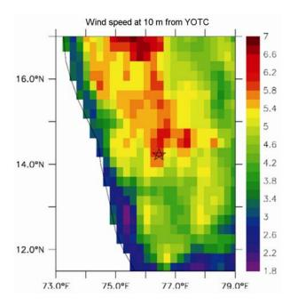
**Figure 7.** Monthly mean wind speed at 10 m above ground for July 2008 from YOTC/ECMWF analysis. The star is the location of the wind farm.
