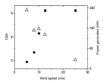
**Figure 6.** Variation of tip speed ratio (TSR;  $\Delta$ ) and power generated ( $\blacksquare$ ) by WEGs as a function of wind speed.
