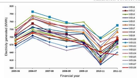
**Figure 2.** Graph of electricity generated by the 18 wind electric generators in each financial year from 2005 to 2011.
