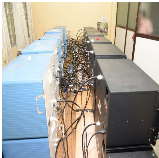
Figure 2: Photograph of the Aethalometers undergoing calibration and inter-comparison tests as part of the campaign. The instruments are seen in the left panel, while the right panel shows the aspiration of air through the manifold
